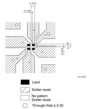
$\mbox{\%}$  Line width to be designed to match 50  $\Omega$  characteristic impedance, depending on PCB material and thickness.
